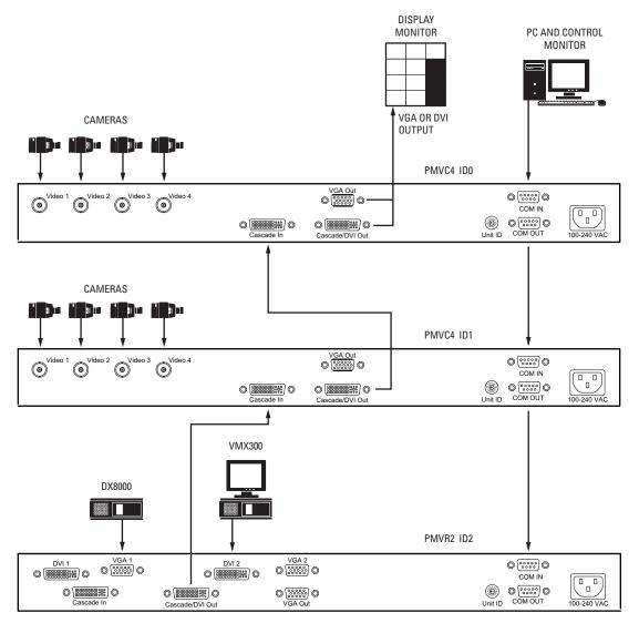
Figure 6. Connecting PMVC4s and a PMVR2
